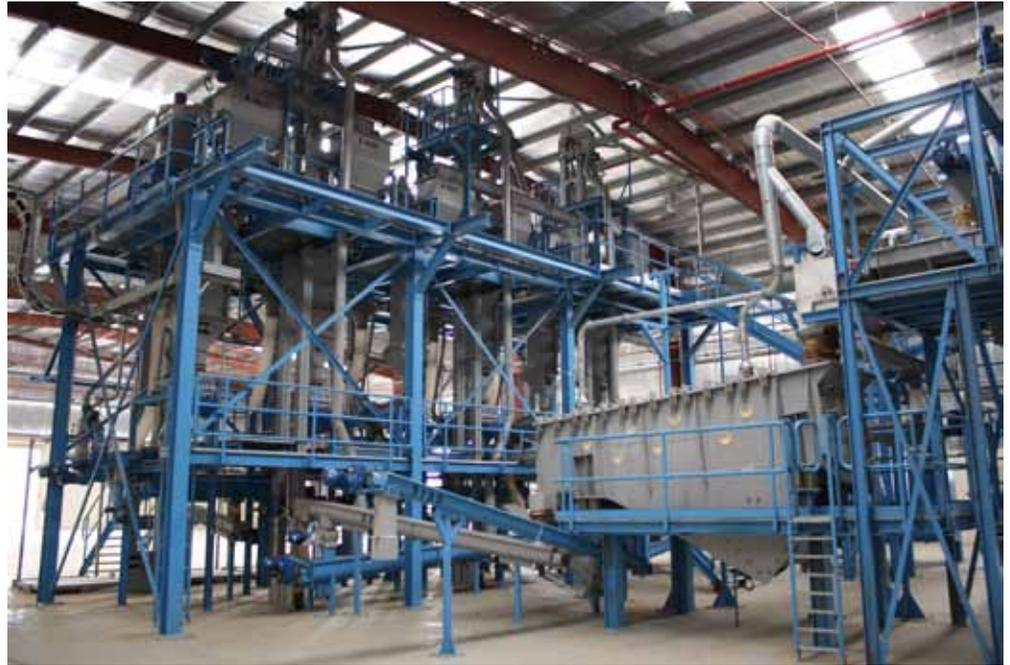
NAW Recycling crumb rubber manufacturing plant
